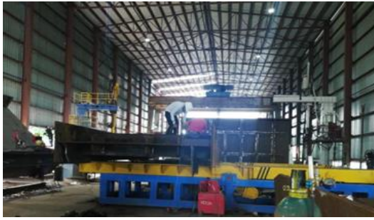
Automatic H Beam Welding Line
