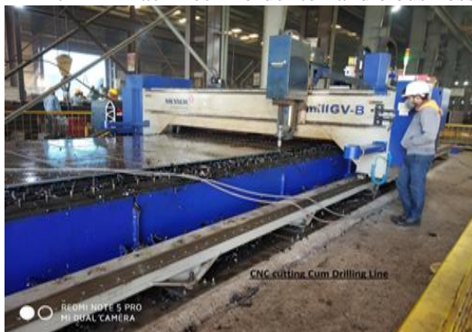
CNC Plamill Cutting Cum Drilling Line
